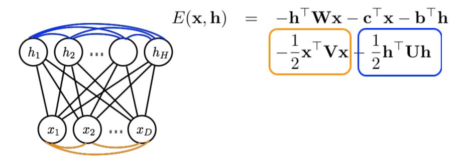
when only one layer has lateral connection, the model is called a  $\triangleright$ semi-restricted Boltzmann machine 50
